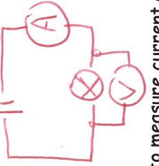
Describe how to measure current and potential difference in a circuit
